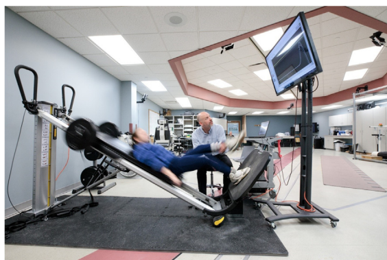
Fig 1 Depiction of a participant in the visual feedback group undergoing power training on the Total Gym GTS system. As shown, the physical therapist and participant viewed a monitor that provided information about the speed of the leg press and the target speed the therapist prescribed for the set.
